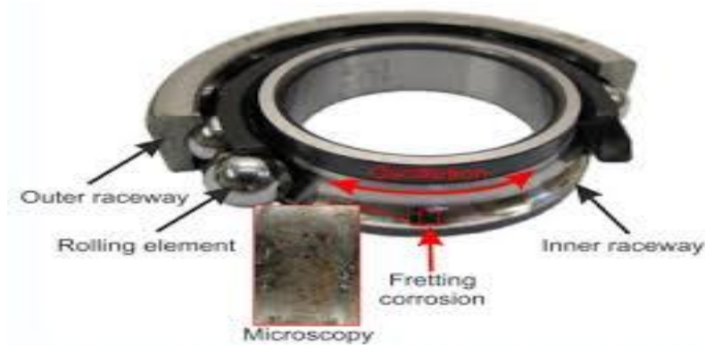
Fig. 2.3: Fretting Corrosion on the inner wall of a ball bearing
