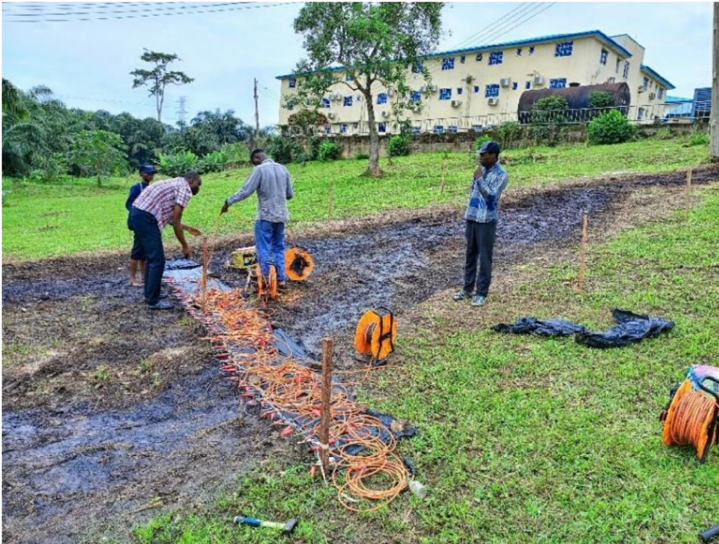
Figure 3.1b Set up of ABEM LS during Data acquisition on Location 2
