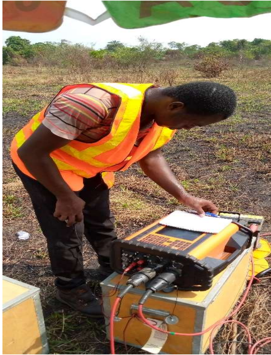
Figure 3.3: Field setup for ABEM Terraloc Pro Seismograph
