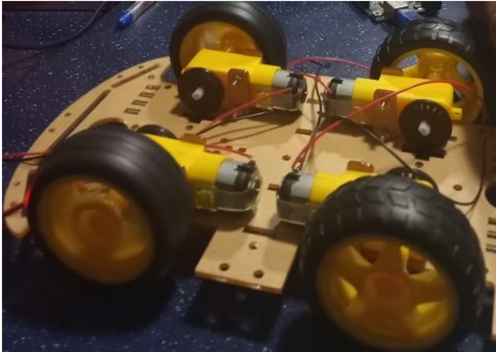
Figure 3.2: Attachment of the motors and wheels to the chassis
