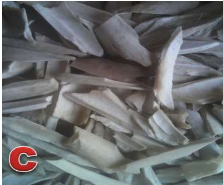
Fig. 1: (a) Raw pig bones, (b) pig bones after treatment with hot water, (c) after deproteinization with NaOH and HCl and (d) synthesized HAp powder at 1000 °C
