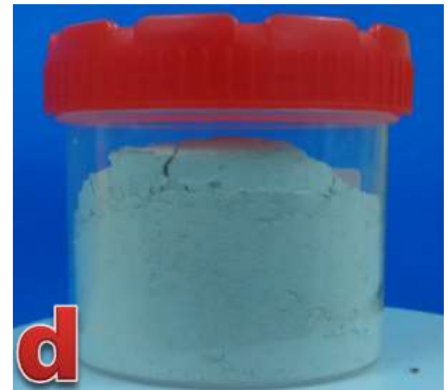
Fig. 1: (a) Raw pig bones, (b) pig bones after treatment with hot water, (c) after deproteinization with NaOH and HCl and (d) synthesized HAp powder at 1000 °C
