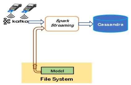
The model will be loaded from the file system via the Spark Streaming Job. After that, it will begin consuming Kafka messages about credit card transactions. This model can be used to determine whether a transaction is fraudulent or not. The forecasts will then be saved to the Cassandra database. Non-fraudulent transactions are saved to a separate table from fraudulent transactions, which are saved to the fraud table.
