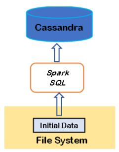
Spark SQL is a Spark module for handling structured data. Thanks to the interfaces provided by Spark SQL, Spark has access to additional information about the data's structure and the computation being performed. Using this extra data, Spark SQL makes improvements internally. (Spark, Sql Programming Guide, n.d.)
