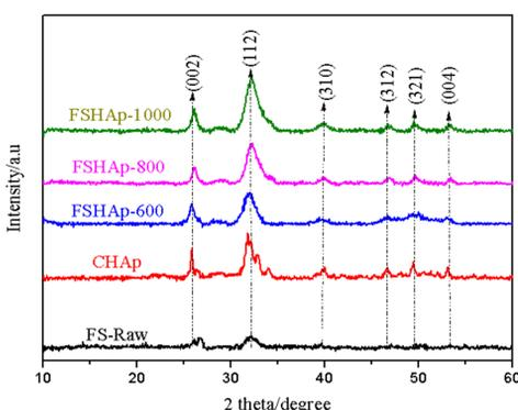
XRD of treated fish scale, commercial HAp and HAp synthesized from fish scales at different temperature
