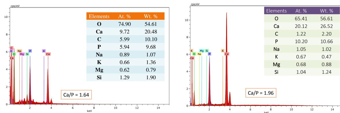
EDX measurement showing the chemical compositions of treated fish scale and HAp synthesized from fish scales at 1000 °C
