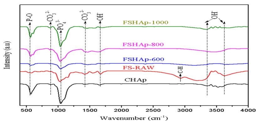
FTIR spectra of CHAp, raw fish scales and HAp synthesized from fish scales at different temperature
