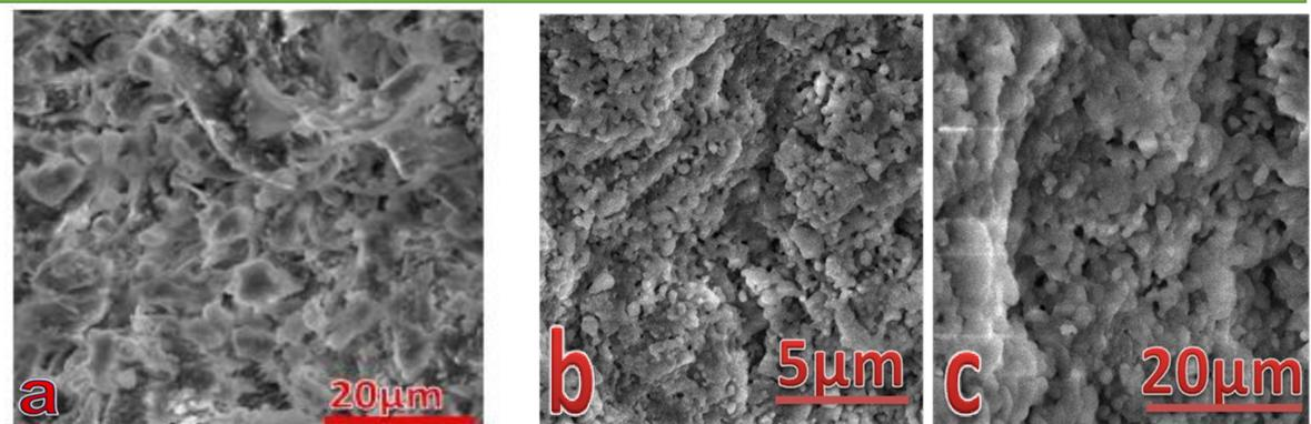
Secondary electron images of (a) FSHAp and (b&c) scaffolds FSHAp
