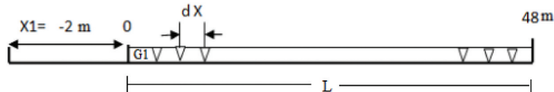
Figure 4. Geometry for MASW data acquisition with array length ( L ) and geophone spacing ( dx ) and forward offset shot ( X1 ).
