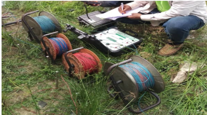
Figure 3. A PASI electrical resistivity metre for 2D resistivity measurements.
